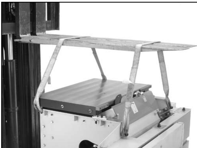
Figure 19. Lifting the saw base unit.
